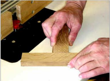
I first wanted to test the bits mainly to see if they were "matched" and if I could change from one bit to the other without resetting router height.
