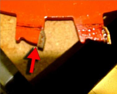
This is a close-up of the teeth with some cleaner on. It shows resin on the edges of the tooth and dirt in between the cutter.
