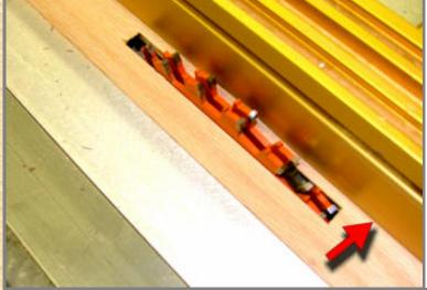
The arrow points to the fence that is overlapping the insert plate. You can see from this view that the "zero insert" should give great cuts.
