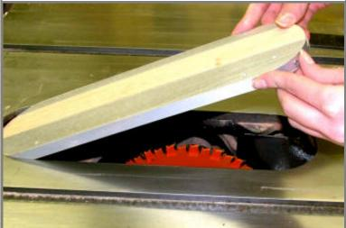
We will take the time to make zero clearance plates for each of the combinations of blades and chipper sets. Joslyn lowers a blank plate so that she can raise the spinning blades through the wood insert. Joslyn has moved the fence so that it is just holding down the plate and raises the blade slowly keeping to the right of the fence so that if the plate came loose, she would not be in the line of fire.
