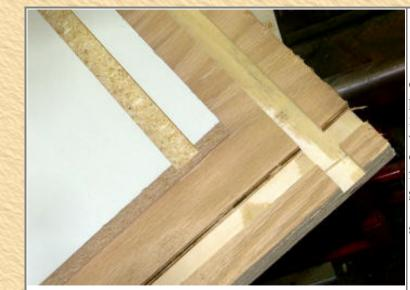
Here are the cuts she made with the full dado set with chippers to make a 3/4" cut. Joslyn made two cuts in the piece of "cheap" birch plywood. There was no tearout or roughness in the bottoms of the dados. Same with the white melamine particle core board — beautiful clean cuts and a smooth groove. Just think of the beautiful, finished dados she would have when plowing cabinet grade plywood and real wood.
