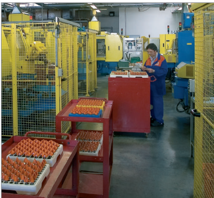
Loading the automated multi-axis CNC sharpening machines.
