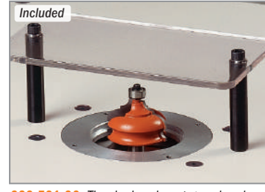
999.501.06 The dual and post-guard makes freehand work safer.
