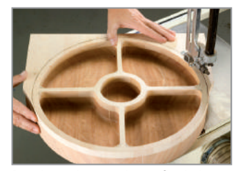
Bandsaw the exterior to final shape.
